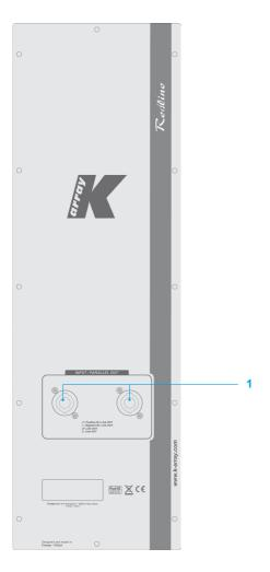
1) INPUT / PARALLEL OUT Speakon connectors. Each connector offers 2 channels of power audio signal. The KMT21P internal wiring is designed to pick up audio power signal from pins 1+ / 1- of a NL4 connector. 2+ and 2- pins, just like 1+ and 1-, are directly wired from one socket to the other, so the signal can pass through multiple speaker modules without additional external cabling.
