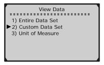
Use the UP/DOWN scroll buttons to move up and down list, and press the Y button to select or deselect data parameters to view. Selected parameters are marked with solid squares.
