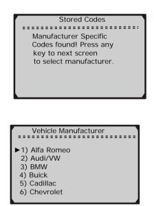
• If the manufacturer for your vehicle is not listed, use the UP/DOWN scroll buttons to select Other and press the Y button.
