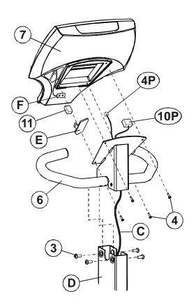
9. Carefully feed the wires back into the top of the CONSOLE SUPPORT ASSEMBLY (#6) and attach the DISPLAY CONSOLE (#7) to the CONSOLE SUPPORT ASSEMBLY using the four CONSOLE SCREWS (#4) and a Phillips screwdriver. Tighten the four SCREWS in a criss-cross pattern.
