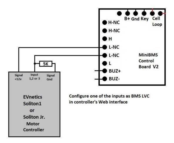
**Auxillary 12V battery note:** MiniBMS relies on constant power supplied from your 12V aux battery. Please make sure your 12V battery is properly charged at all times to ensure correct BMS operation. For safety reasons MiniBMS will shut off the charging process if it loses 12V power to the head end control board, which may leave you with undercharged pack unexpectedly.
