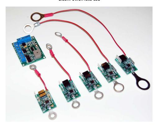
MiniBMS is a battery management system designed for LiFePo4 cells, used in Electric Vehicles. MiniBMS is designed to be reliable and cost effective solution; it has most basic functions, implemented via simple one wire interface, which also allows easy installation and troubleshooting.
