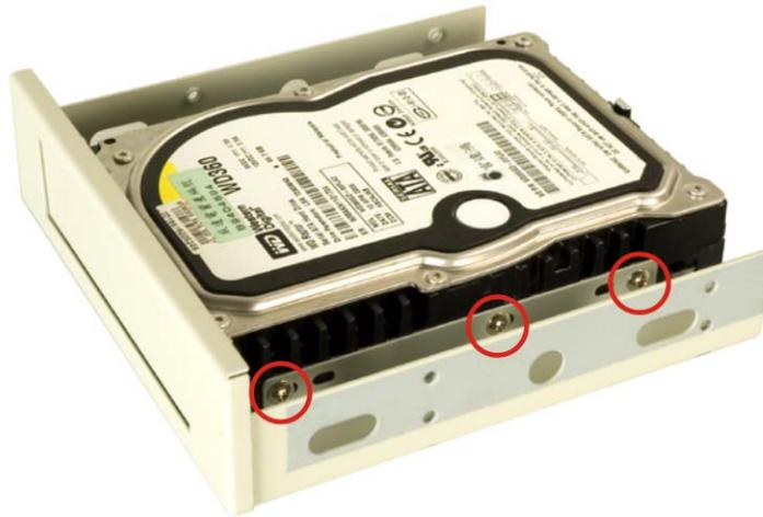
Figure 4-9: 3.5" to 5.25" Drive Adapter Bracket Retention Screws
