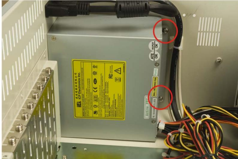
**Figure 5-2: PSU Internal Retention Screws**
