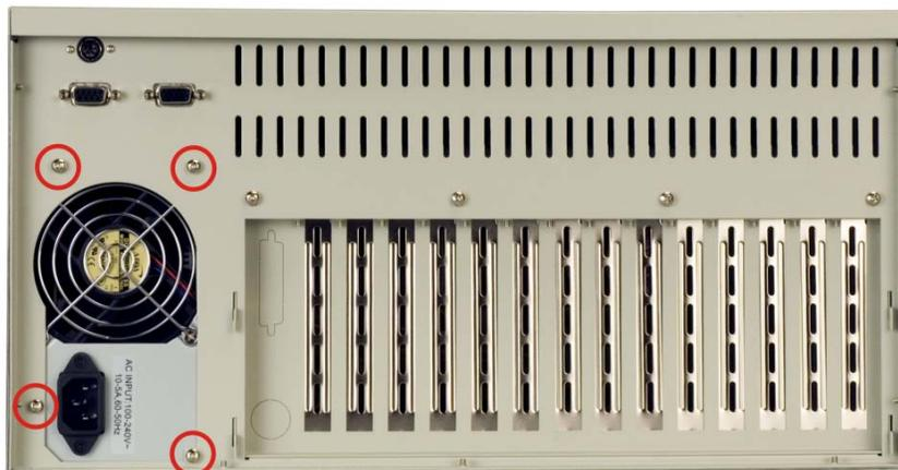
**Figure 5-1: PSU External Retention Screws**
