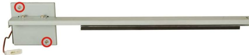
**Figure 5-3: System Fan Retention Screws**
