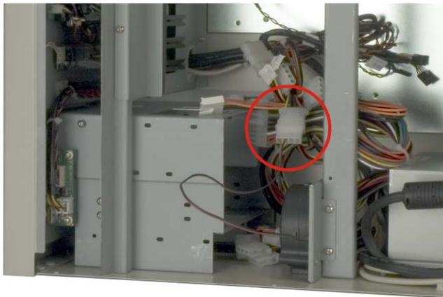
Figure 4-4: Detach the System Fan Power Cable
