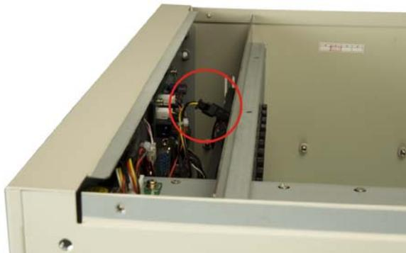
**Figure 5-4: Disconnect the Cooling Fan**
