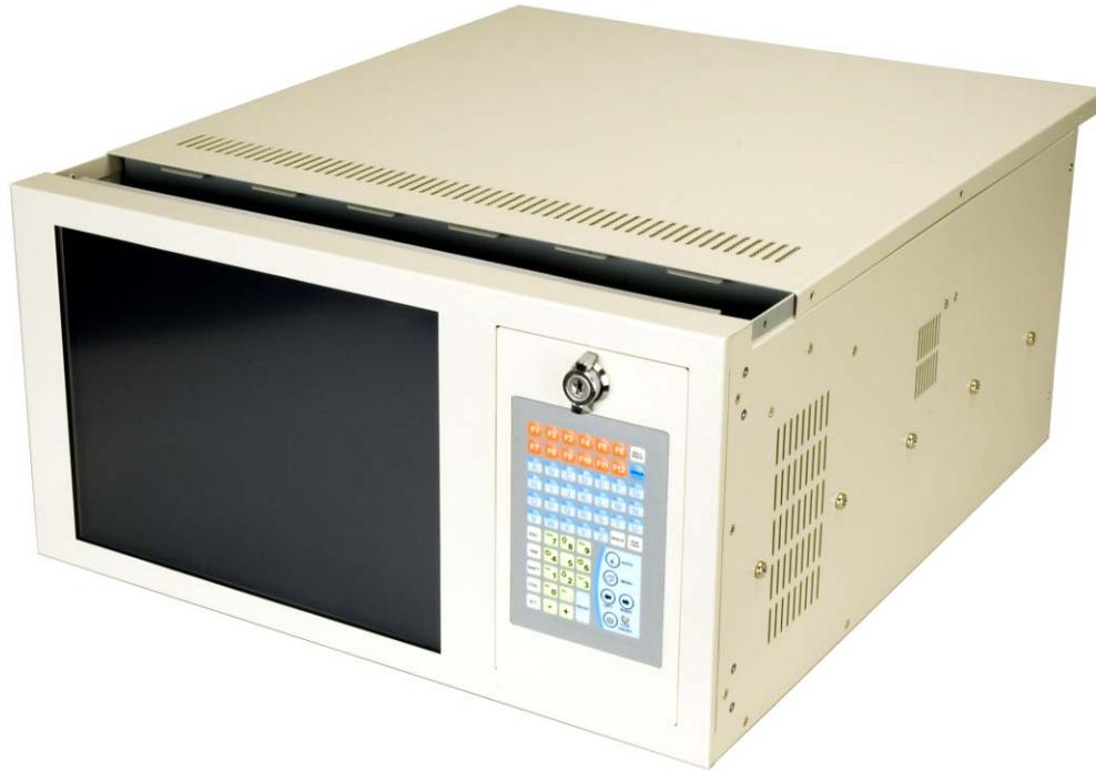
**Figure 4-2: Remove the Top Cover from the Chassis**
