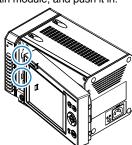
4, Join the display module with the module connector, and insert into the main module.
