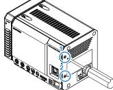
2, Pull the nail on the upper-right side of the face cover, and remove the face cover.
