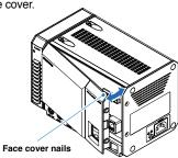
3, Join the nails on the back of the display module with the inset part of the main module, and push it in.
