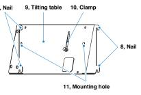
8, Nail...... Nails for fixing to the main module (4 places)
