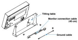
1, Install by binding the monitor connection cable with the clamp on the tilting table.
