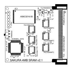
Revision 2.x Sakura boards are built around Alliance Memory AS6C3216, which is a 55ns 32 megabit SRAM chip with 16-bit data bus. The memory is accessible within high 4MB of Zorro 2 memory (0x600000-0x9FFFFF) range.
