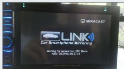
FIG.2 Press switch button once to switch to Miracast PBC mode (screen mirroring)
