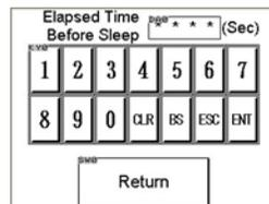
Enter the desired elapsed time before sleep mode in seconds on the keypad touch screen.
