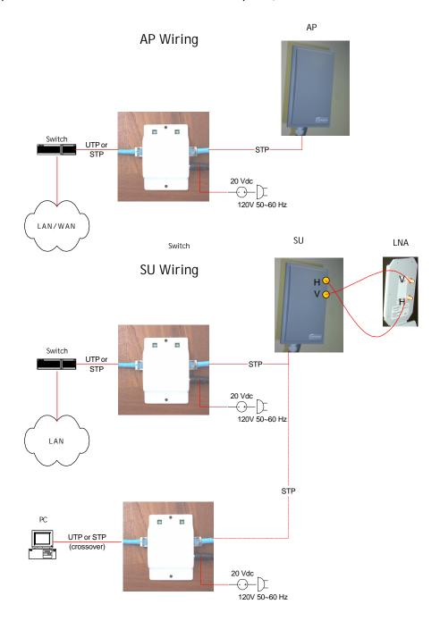
The maximum cable length from the Junction Box to the unit (AP or SU) is 100 meters (328feet). Please note that the maximum cable length from the radio to PC/hub/switch is 100 meters (328 feet), as specified in the Ethernet standard.
