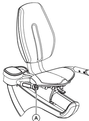
At-Your-Fingertips Resistance Controls are located on the right armrest and right side handlebar on the Recumbent Lifecycle Exercise Bike.
