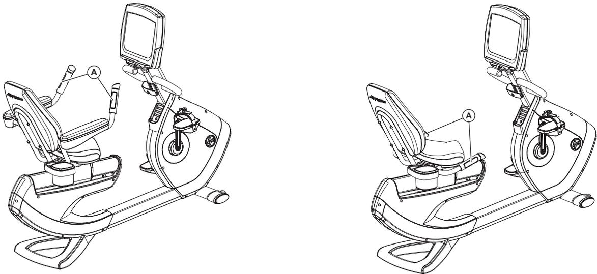
Grasp the sensors that are located on either the armrests or the side handlebars of the Recumbent Lifecycle Exercise Bike.
