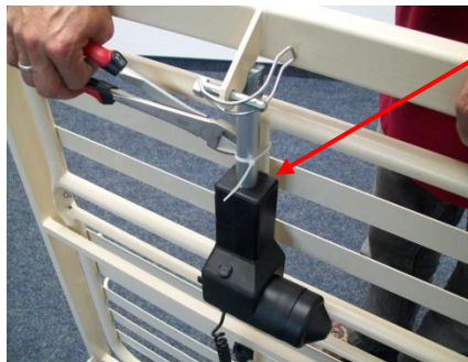
Thigh rest adjustment motor
