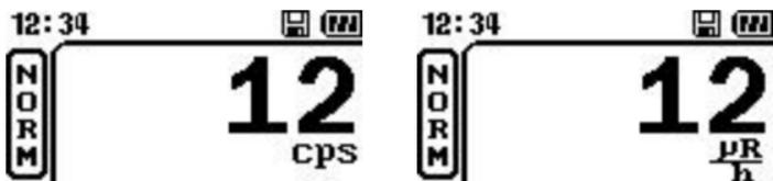
When Stay Time is less than two hours, the display alternates between Stay Time and Dose Rate:
