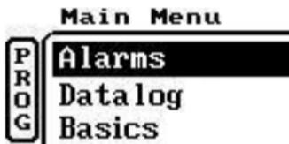
Press the MODE button to step through the menu of parameters. Press the SET button to select a parameter.
