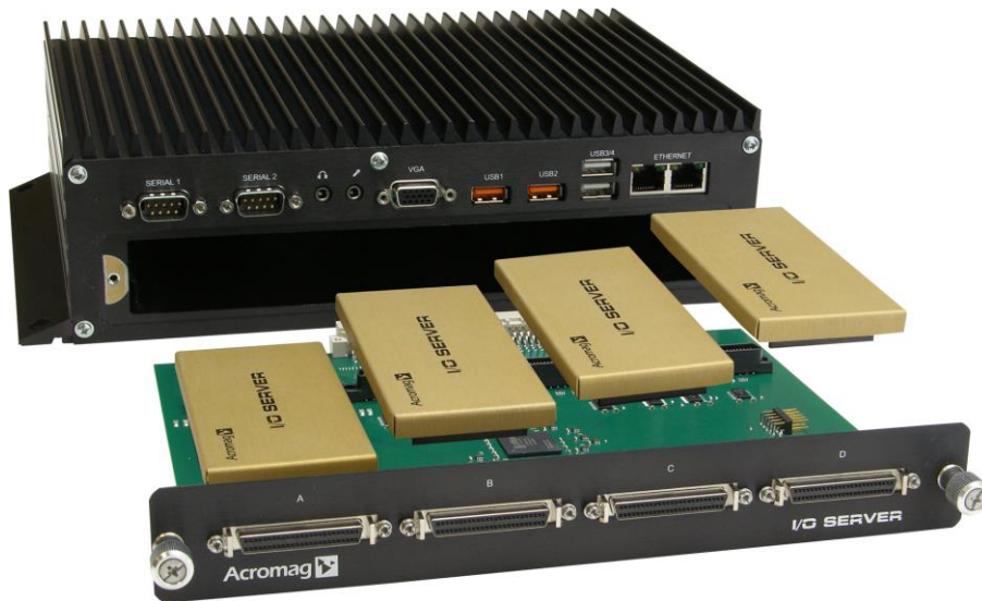
Figure 2.2a: IOS Module Installation
