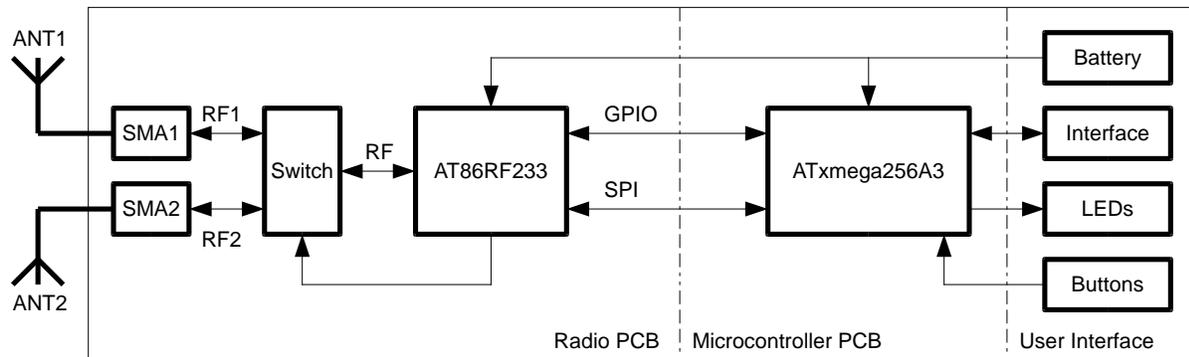
The two REB233CBB Module components, the Radio PCB, equipped with two swivel antennas, and Microcontroller PCB, are shown in detail in Figure 5-2. Here, the REB233CBB Module is dismantled for better explanation of all important hardware features.
