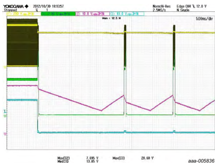
a. Output short circuit during normal operation
