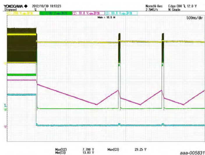
a. Output short circuit during normal operation
