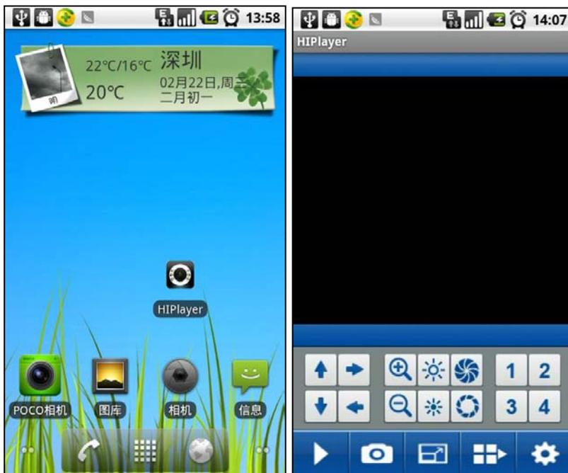
3. Click the button
