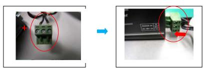
5) Connect the power cord to the power adapter and then connect the plug of the adapter to the multi tap cord located at the back side of the sub-rack. Finally, tidy up the power cables using the cable ties.
