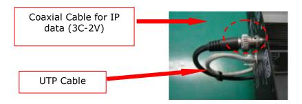
\*\* Precaution: Please be careful when connecting the BNC connector. If you apply too much force to the BNC connector of the receiver, it may damage the BNC connect port.
