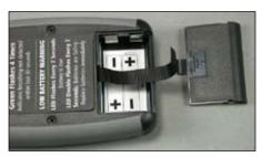
Figure 29 **OPC Batteries Removed**
