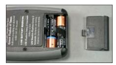
Figure 28- OPC Back **Battery Cover Removed**
