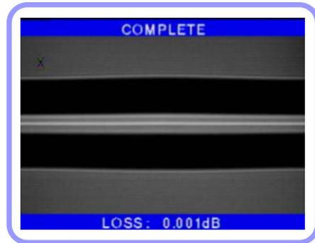
If the measured cut angle or computed loss value is greater than the preset limit, an error message appears on the screen. Also, an alarm can be triggered by the discovery of an abnormal condition of the spliced part including too thick or thin area or bubbles. Even if an error message does not occur, it is recommended to perform the arc fusion process again if the result on the screen does not look good enough when examining it with naked eyes.
