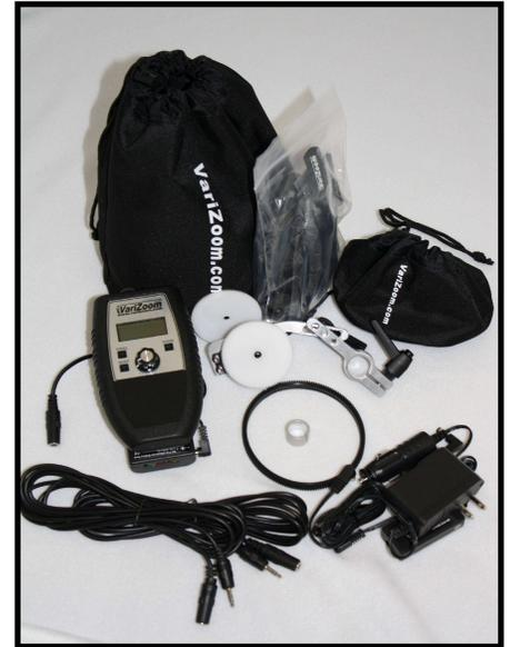
First, determine which gear you need to use and attach it to the motor. The Canon gear is marked "C" and the Fujinon is marked "F". Sony EX series of cameras use the "F" gear and others use "32" gear. 1) Remove the screw in the center of the motor spindle. 2) Install the appropriate gear. 3) Replace the screw in the motor spindle.
