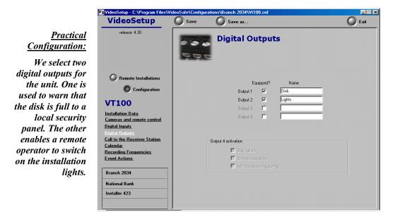
Fig. 22 - VT100 Digital output configuration folder
