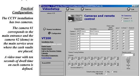
Fig. 50 - VT200 Cameras configuration folder
