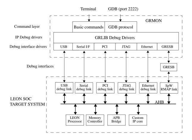
GRMON can operate in two modes: command-line mode and GDB mode. In command-line mode, GRMON commands are entered manually through a terminal window. In GDB mode, GRMON acts as a GDB gateway and translates the GDB extended-remote protocol to debug commands on the target system.
