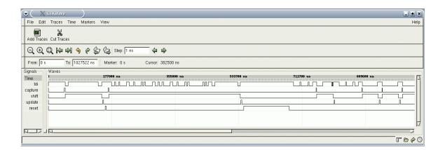
To simplify the operation of the logic analyzer, a graphical GUI is available. The GUI is written in Tcl/Tk and can be connected to GRMON using the GDB interface. To use the GUI, enter the gdb command in GRMON and then launch the tcl file logan.tcl.
