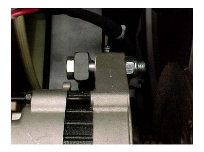
4. Use the 5/16 hex bolt supplied in the kit and with the existing Alternator Mounting bolt, fasten the Shroud Support Bracket to Alternator and tighten the bolts.
