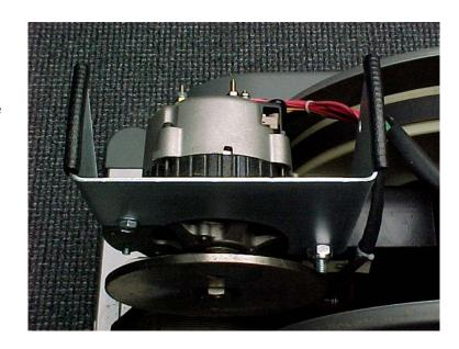
Use top hole on Alternator \_ to mount Support Bracket
