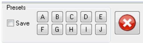
To stop the traverse, click the Stop Motion button
