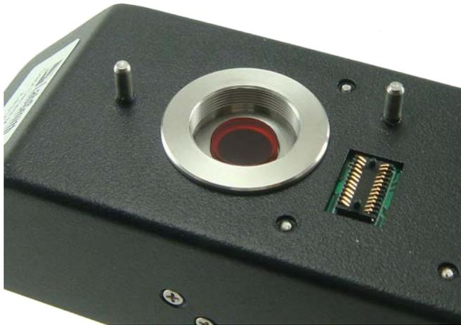
*Fluorescence filter installed in an optics module; note: filter washer is placed on top of filter*
