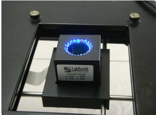
*Illumination module installed in SVM340*
