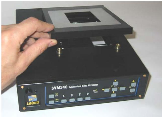
*Removing the microscope stage*
