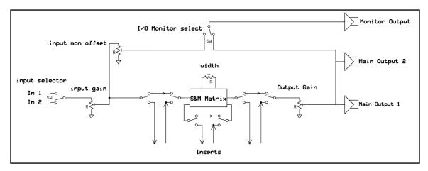
An analog source is fed to the input where the input gain control lets one precisely set the level and balance into the insert stack.
