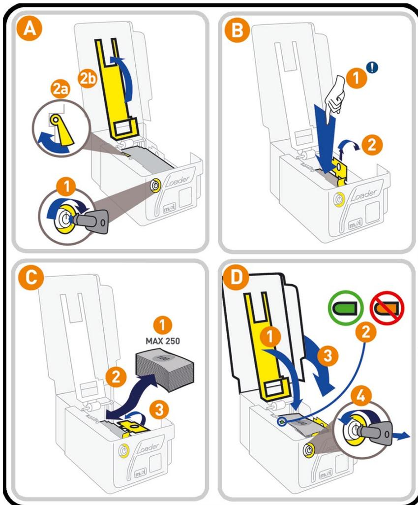
Reposition the “max level detection plate”.
