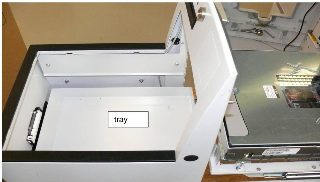
Reinsert the tray after cleaning. Push the scanner completely to the front and close the device.
