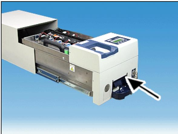
Push the coin module into the housing as far as possible.
