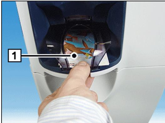
Notes that show irregularities during feed and notes that are not recognized (potential forgeries) are routed to the reject/cash output tray (1) without the deposit process being interrupted.
