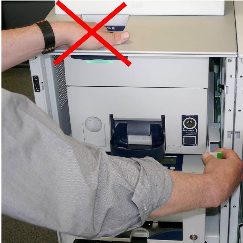
Grasp the module only at the green lever and pull it out to the service stop (approx. 20 cm).
