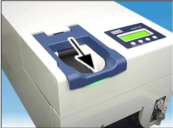
Release the blue faceplate of the coin entry tank via the product-specific software and push it in the direction of the arrow as shown here and ...
