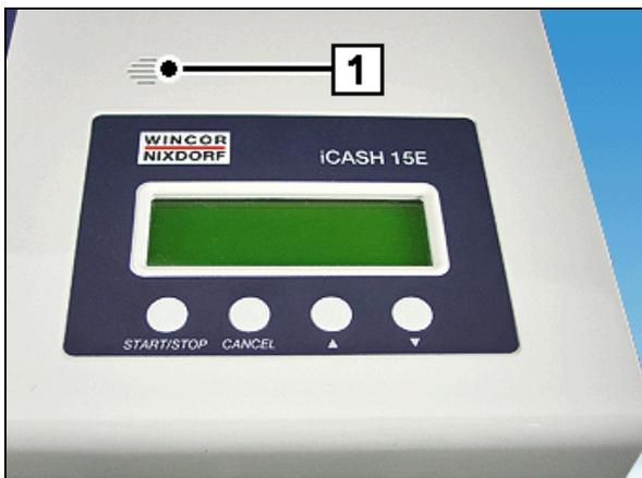
Acoustic signals are output over the loudspeaker (1).
