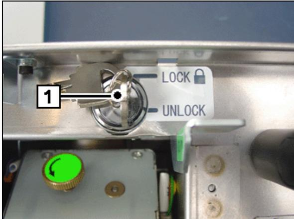
Insert the key used to unlock the coin module (key 2 in the section "Keys for iCASH 15E") in the lock and turn it to the left until it reaches the 'UNLOCK' position.
