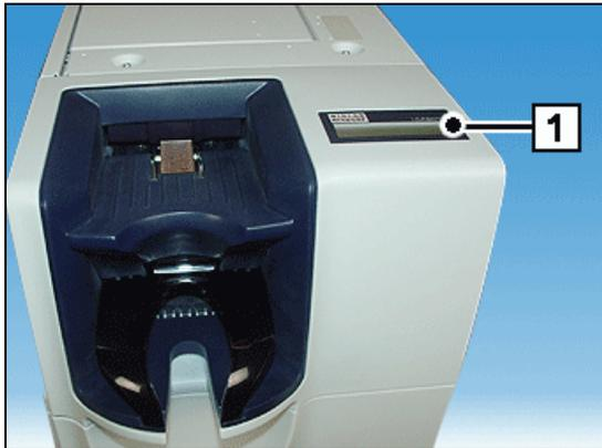
Any malfunctions are signaled to the application by the controller and displayed on the operator display (1).
