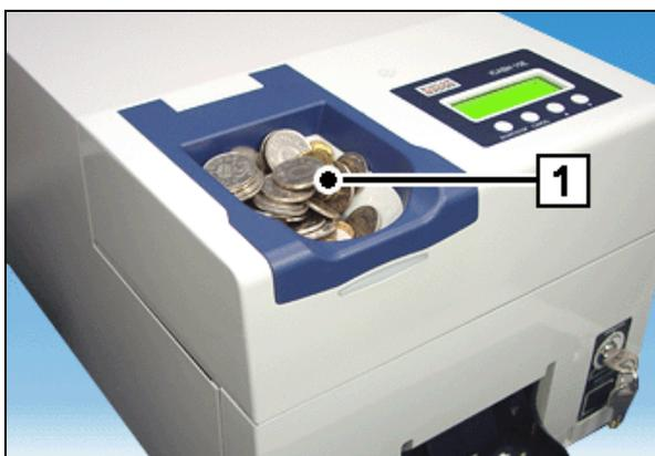
Place the coins in the coin entry tank (1) and start the deposit process via the product-specific software.
