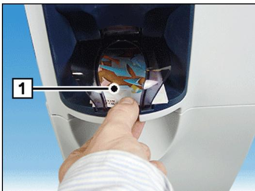
Banknotes totaling the required amount are stored in the reject / output tray (1).
