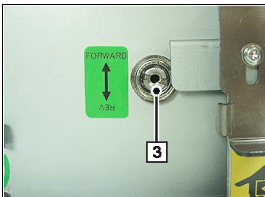
... uncovering the service hole (3) on the drum module.
