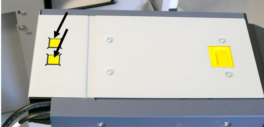
...and open the recognition sensor door. Withdraw the banknote and close the sensor again.
