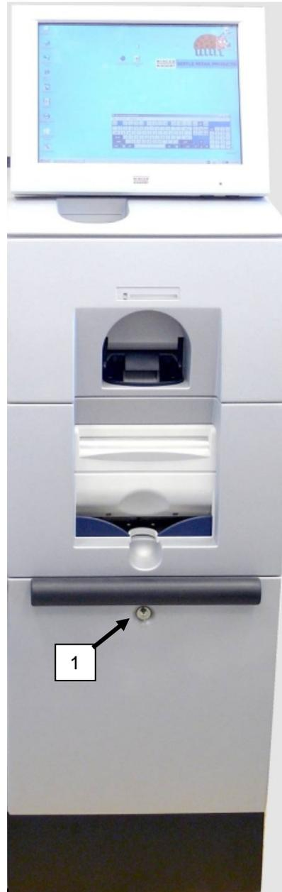
To open the safe, enter the code (1), turn the lock/unlock handle clockwise (2) and open the door.
