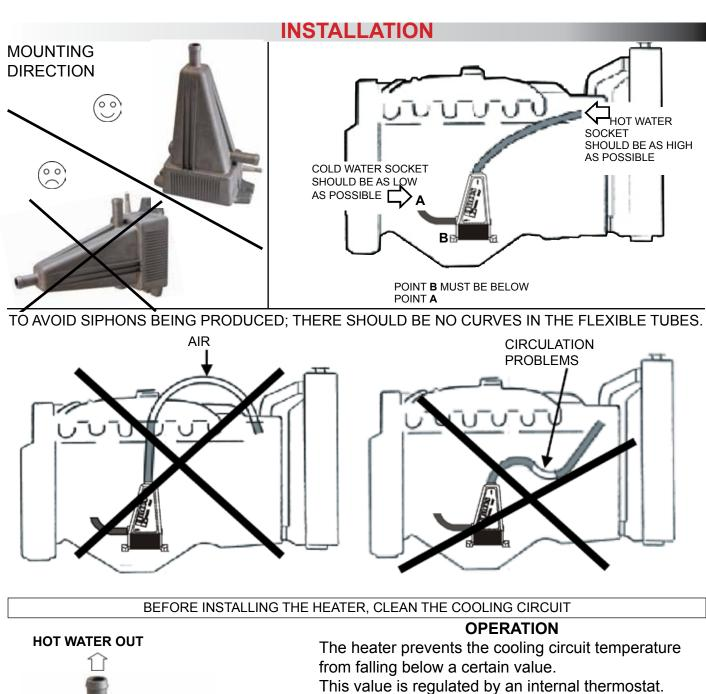
The water circulates using the thermosiphon principle.
