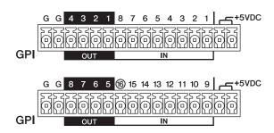
The MTX5-D provides 16 input ports and 8 output ports.
