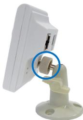
2. Adjust the angle of the camera based on live view.
