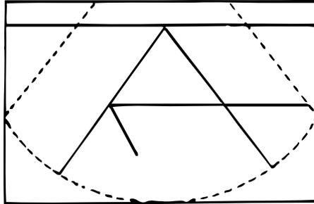
Plywood marked as shown and cut on dashed lines
