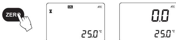
4. Gently absorb the ZERO water standard with a soft tissue. Use care not to scratch the prism surface. Wipe off the surface completely. The instrument is ready for sample measurement.
