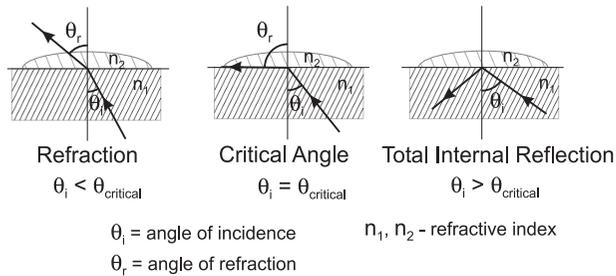
In the HI 96801, light from an LED passes through a prism in contact with the sample. An image sensor determines the critical angle at which the light is no longer refracted through the sample. The HI 96801 automatically applies temperature compensation to the measurement and converts the refractive index of the sample to sucrose concentration in units of percent (by weight) Brix.
