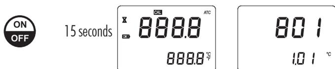
2. While continuing to hold the **ON/OFF** key, press the **ZERO** key. The temperature unit will change from °C to °F or vice versa.
