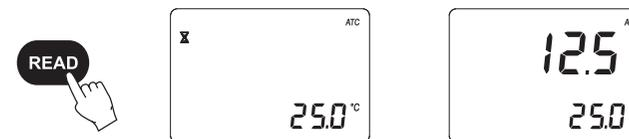
**Note:** The ATC tag blinks and automatic temperature compensation is disabled if the temperature exceeds the 10-40°C / 50-104°F range.
