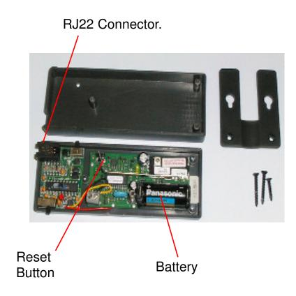
Remove the old battery from the battery holder and place the new battery with the positive end of the battery facing up towards the bottom of the unit towards the RJ22 connector. BE SURE TO PRESS THE RESET BUTTON AFTER INSTALLING THE NEW BATTERY.
