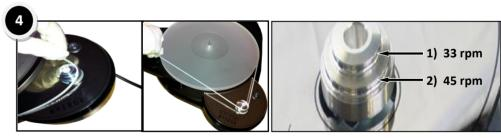
Remove the Drive Belt and gently place it around the platter and then onto the pulley. Note position 1 is for 33 rpm and position 2 is for 45 rpm. It is important to check that your mains supply frequency corresponds to the frequency specified on the Radius5 MkII mains input label.
