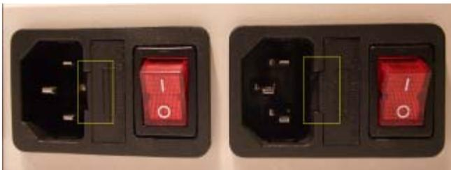
2.) Carefully remove the fuse holder with a flat screwdriver.
