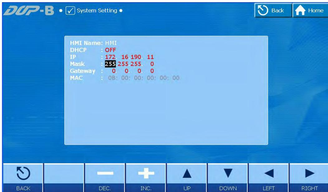
After completing all the settings and make sure that the communication is good, use the most updated Screen Editor program editing software to open the selected .dpb file which just has been modified on eServer. Create a character input element and set its address to \$100.
