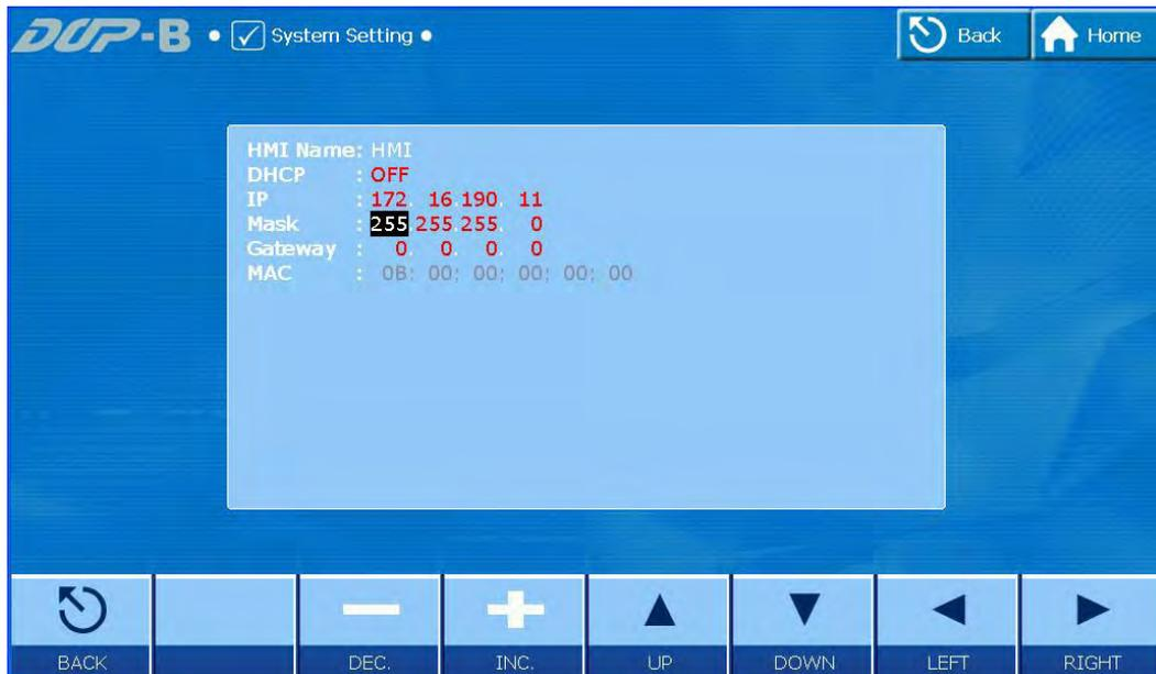
After completing all the settings and make sure that the communication is good, use the most updated Screen Editor program editing software to open the selected .dps file which just has been modified on eServer. Then, create two elements. One is a character input element and its address is set to \$100. The other is a maintained button element and its address is set to \$0.0. Please refer to the figure below:
