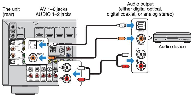
If you select the input source by pressing AV 1-6 or AUDIO 1-2, the audio played back on the audio device will be output from the unit.
