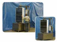
Each bundle is then placed on the bottom plate which has been specifically designed for screens. The top platum, which is also designed specifically for screens, is then lowered and the variable speed drive takes over.
