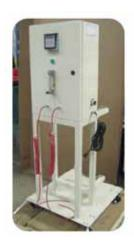
The range of the machines comprise of the new basic Multi-1, which can be used with all gases, but is especially designed for use with Krypton, Zenon and SF6, with a gas flow rate of 10 to 12 liters per minute.
