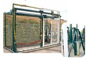
It uses both horizontal and vertical clamps to hold the frame in place. With the fixed member locked in with scissors, attaching the movable panel becomes simple and allows for testing.
