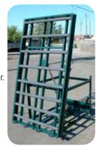
a window dolly for easy transport to the shipping area. As with all roller conveyers, the rollers are non-marking for use with vinyl, wood or aluminum. Oversized cylinders for heavy windows and closer roller spacing are a couple options to consider.
