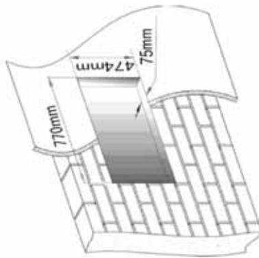
2. Create a channel within the wall below the TV recess, which allows the cables to drop into. Channel width: 50mm.
