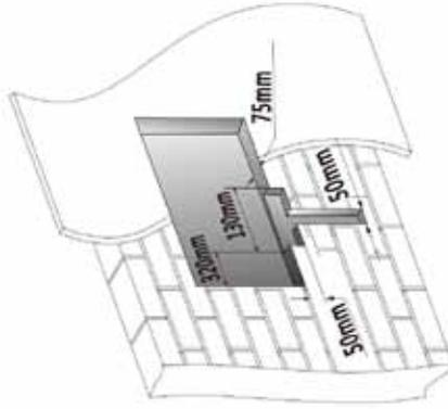
3. Place the in-wall bracket into the recess and use the 4 x pilot holes to drill into the wall. Place the 4 x raw plugs into the holes that have been drilled and screw the bracket into position.
