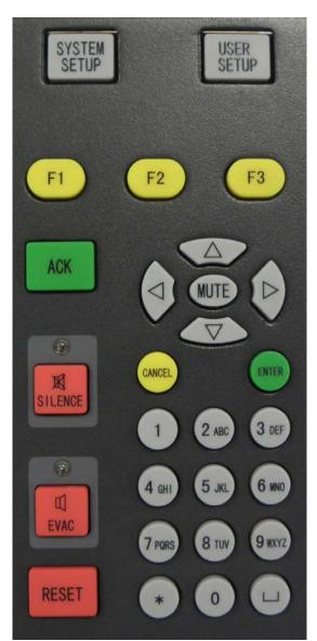
**SYSTEM SETUP:** The System Set-up button is used to access to the system menu. Each option in the menu corresponds to one number button. This is accessible under the manager password.
