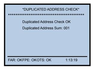
If the system found the devices with duplicated address, the total number will be displayed. To find the exact addresses and loop location press **USER SETUP** button and select **1 BROWSE** then select **4 BROWSE DUPLICATED ADDRESS**
