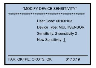
The system verified the existing device sensitivity **ENTER.**
