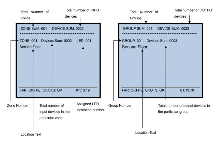
To view the list of devices that are belong to a particular zone, select the zone using the arrow cursor **UP or Down** and then press **Enter**.
