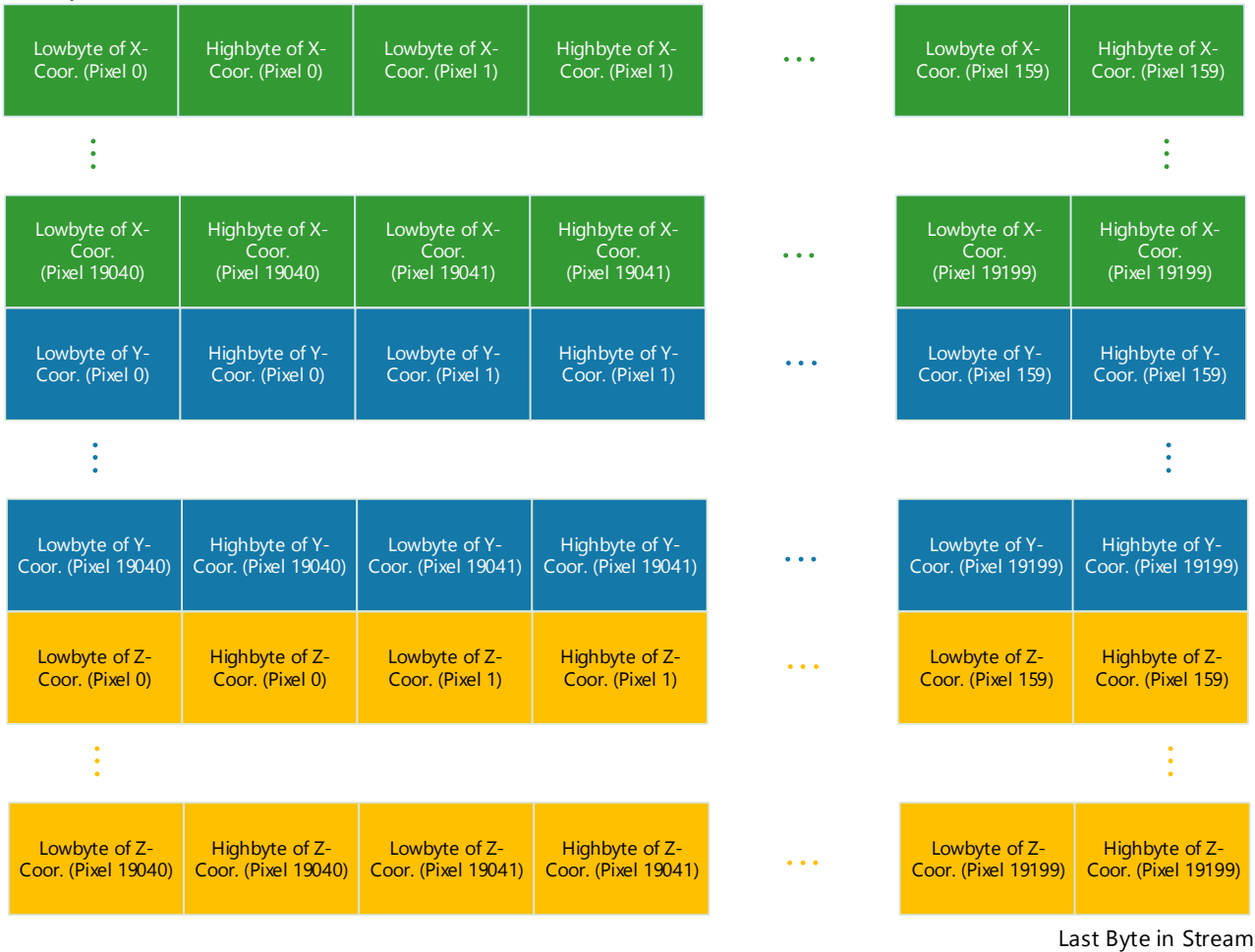
Figure 4-4: Data stream of XYZ Point Cloud
