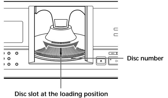
The disc number at the loading position appears in the display. If the disc has the Disc Memo (see page 18), the Disc Memo appears instead of the disc number. As you turn the JOG dial, the disc number or the Disc Memo changes.
