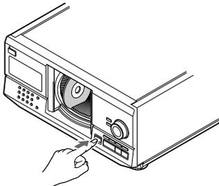
The rotary table turns and the disc slot at the loading position is set to the playing position. Always close the front cover except when you insert or remove discs.
