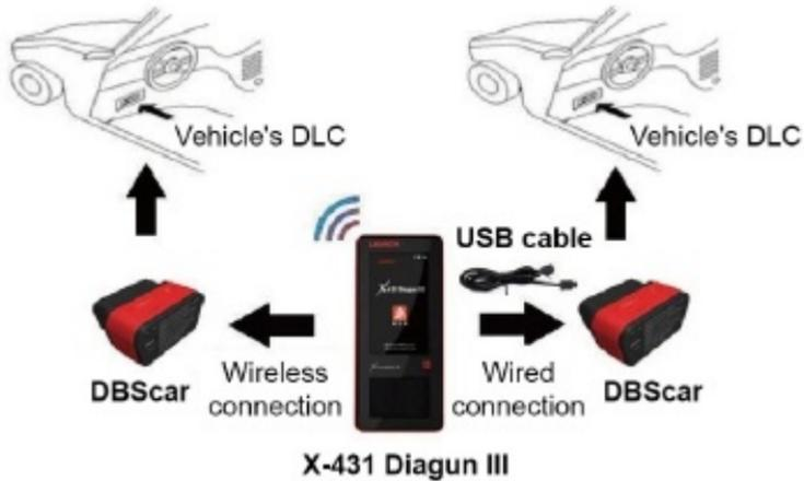
Fig. 3-2 Bluetooth (wireless) / Cable (wired) connections
