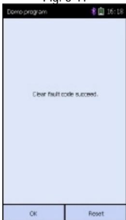
"Clear fault code succeed" will appear if succeed (See Fig. 3-12), or "No fault code" will appear on the screen if all the fault codes have been cleared or no fault code in the tested system.
