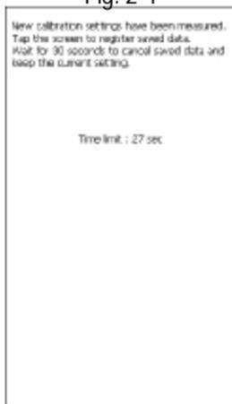
After calibration, the screen will display as Fig. 2-5. Touch the screen to save your calibration and enter the main menu. To exit without saving your changes, wait for 30 seconds and the system will cancel it.
