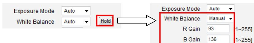
For advanced users, there is also an option to switch from Auto mode to **Manual mode** of White Balance directly and input the R Gain and B Gain values manually.
