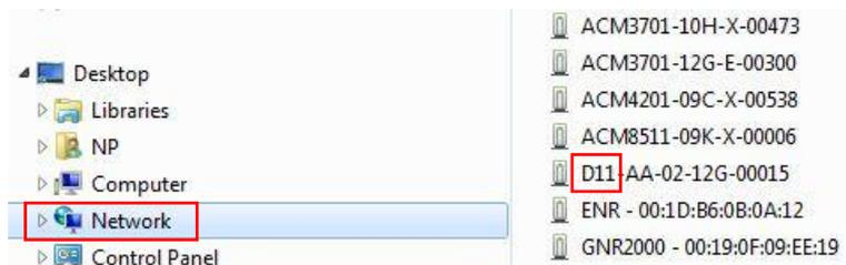
With the left mouse click on D11 it is possible to automatically launch the default browser of the PC with the IP address of the target camera filled in the address bar of the browser already.
