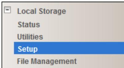
The "Setup" function provides the option to manage the file writing behavior of the camera. By default, the camera is set to "Remove old recordings when ran out of storage space automatically". By using this mode, the camera's recording process will not be interrupted when the disk becomes full – the oldest files will be overwritten by new recordings.
