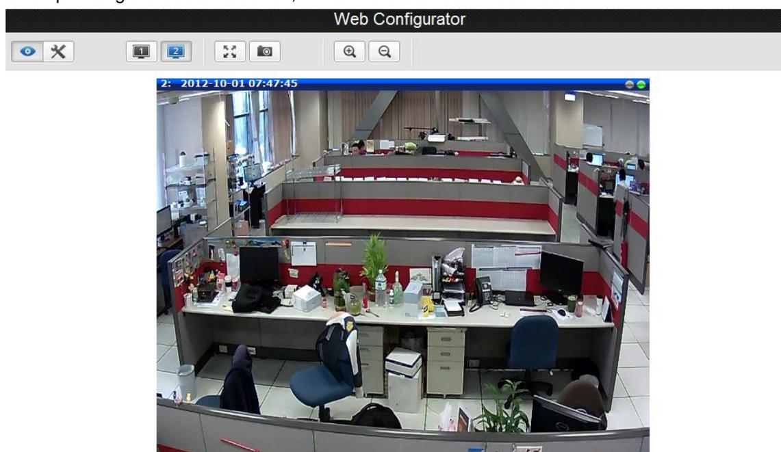
To capture the snapshots of the current live view, press the snapshot button. The snapshots are saved in Pictures folder.
