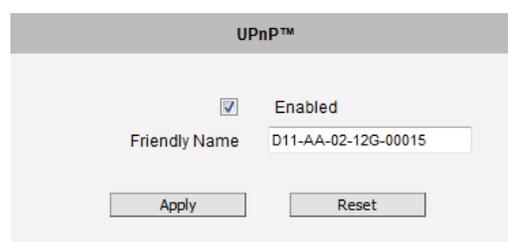
The **Friendly Name** is a human-readable name for the device that will be displayed when the camera is found. By default, the serial number of the camera is used as a friendly name; however, the user can modify the name according to the project needs.
