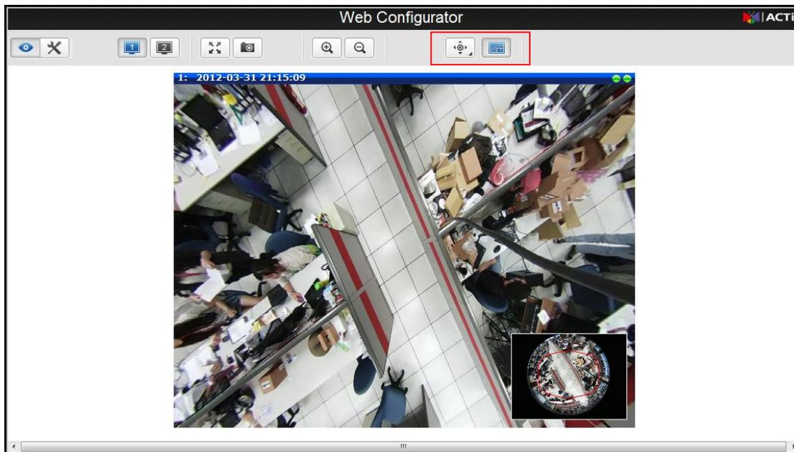
By default, a miniature of the Fisheye view is shown on the lower right corner of the Live View,
