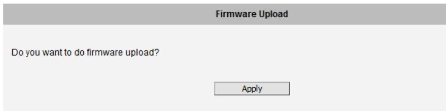
After pressing **Apply** button, it is possible to browse for firmware image file that has already been downloaded to the computer that has the Web Configurator running.
