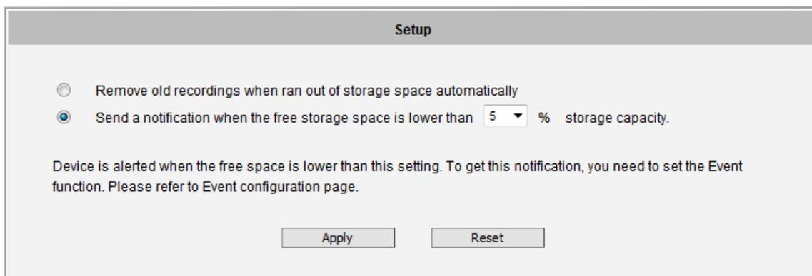
By this option, the possibility of sending notification e-mails automatically has been enabled. The % refers to the remaining size of available storage at which the camera should send a notification e-mail, in case such task has been listed in Event Handler of the camera. To actually make the e-mail notification work, please go to Event Handler (See “Event Handler with Local Storage” on page 101.) of the camera and set up the event rule where the selected trigger type is “disk space is low”.
