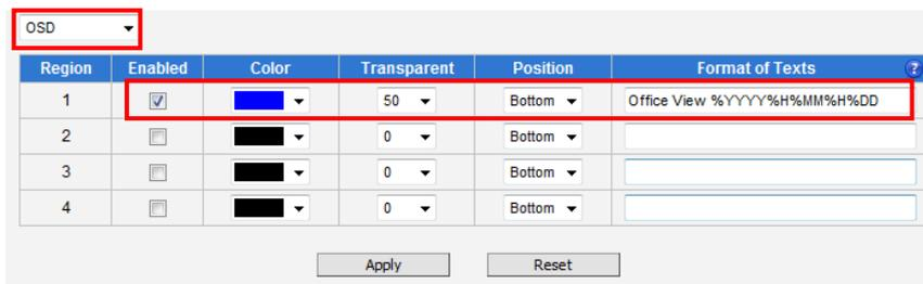
In the example above, one region of text was enabled with blue color and 50% transparency, located at left lower corner and containing the text of "Office View" together with current date. The date would be automatically changing every day, according to camera's date and time settings. The result of the example configuration would look like this (Live View page, 1:1 scale):
