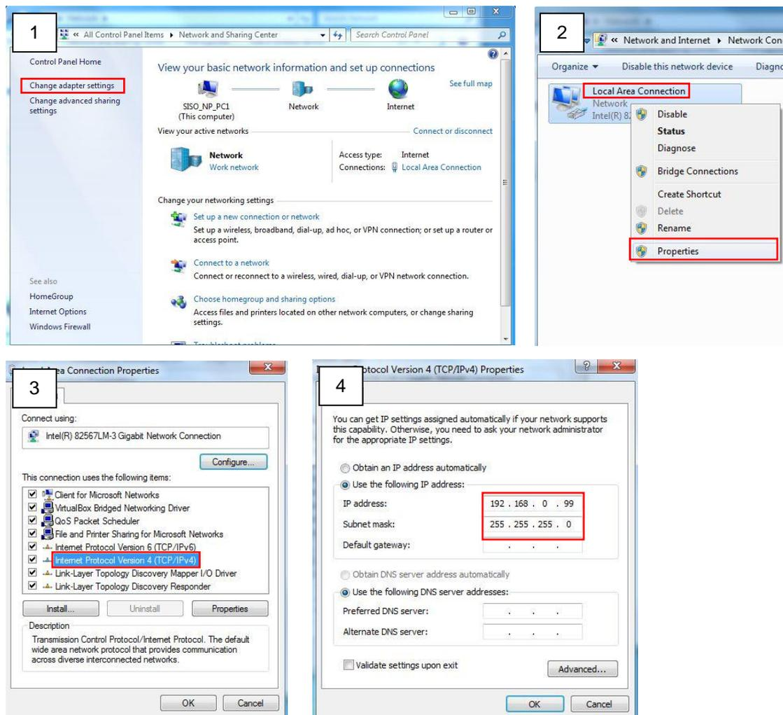
**Manually adjust the IP addresses of multiple cameras:**
