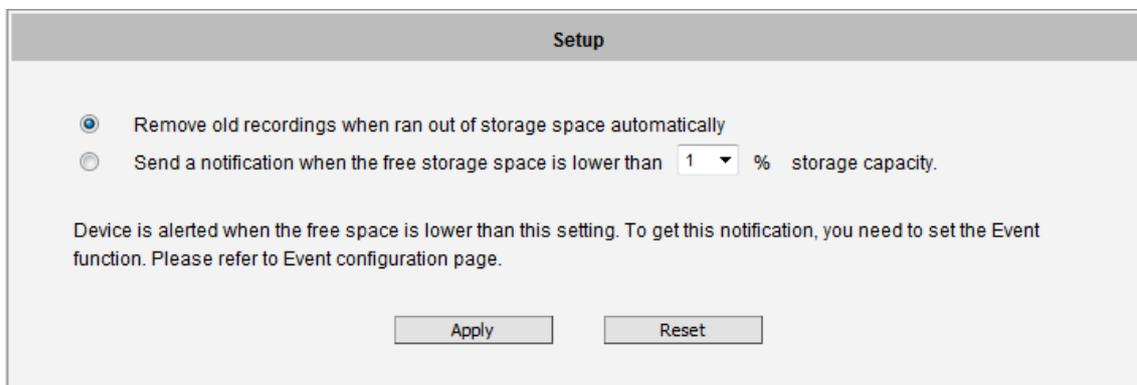
Please note that under this mode, there is a risk that important evidence may be deleted automatically over a period of time. Therefore, as long as "recycling" mode is used, the user should download the critical evidence files from the camera before they are erased by the camera.
