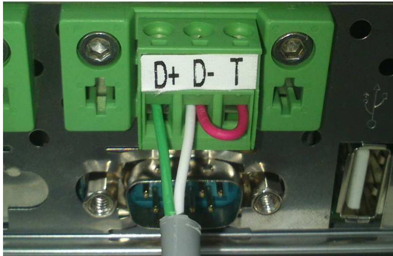
Figure 4 - Built-in RS485 with internal termination activated (bridge between the terminals D and T). If you do not want to use the termination do not bridge the terminals
