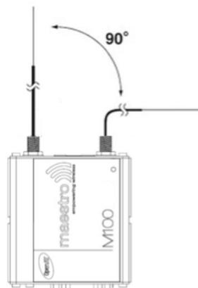
Figure 2: Antenna positions
