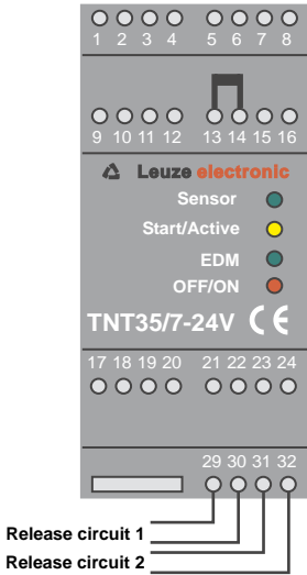
Figure 5.9: Wiring safety output (two-channel release circuit)
