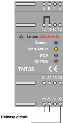
Figure 4.8: Wiring safety output (one-channel release circuit)
