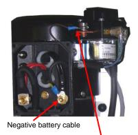
Positive battery cable. Please connect a fuse holder to this cable.
