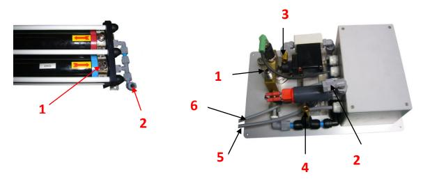
The control panel must be mounted on a vertical surface as close as possible to the motor / pump unit and to the membranes. Leave space behind the panel to facilitate the connections. It is recommended that it is installed at the bottom or on the sides of cupboards, under chart table or main cabin seats, on the front panel of a rear bunk, ...
