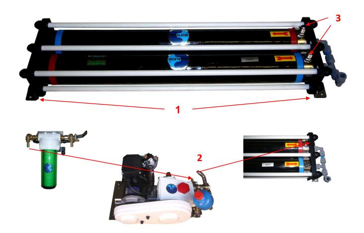
The membranes can be installed horizontally, preferably flat or on a wall support. They are mounted using 8 Parker screws in stainless steel brackets<sup>1</sup>. As the hose from the HP pump<sup>2</sup> vibrates, it is preferable to install the hose with an insulating tube. The HP connectors should be installed strictly in accordance with the instructions (Appendix A2). Apply a little loctite or nut seal to the two male and female cones before tightening.
