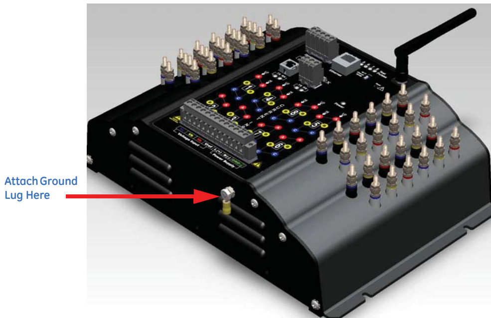
FIGURE 4.1: Ground Lug Connection
