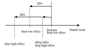
$SD1 = 5^{\circ}C$ ,  $SD2=5^{\circ}C$  and Offset  $SD2=3^{\circ}C$  as default.
